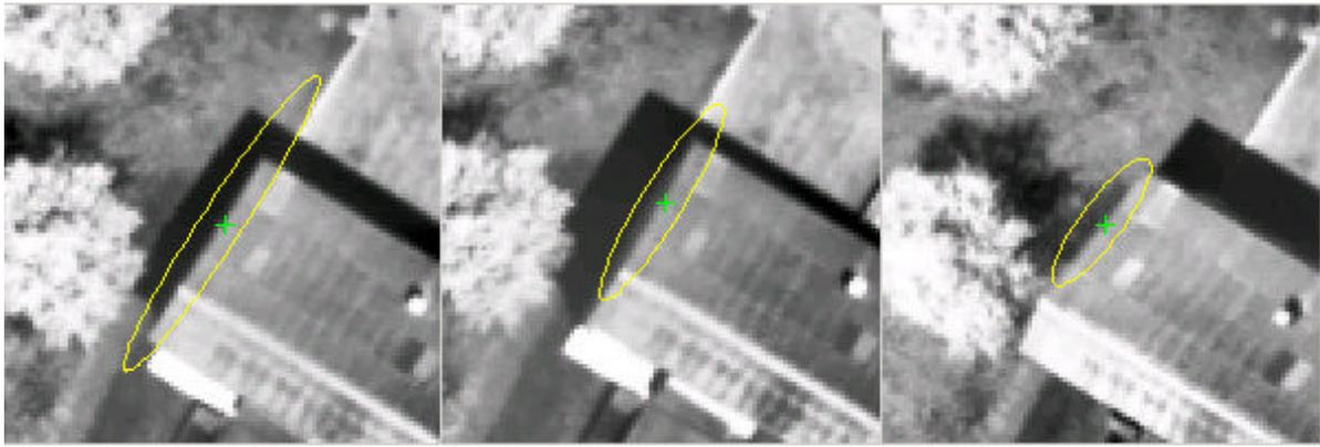
**Figure 5.** On the left, in the middle, on the right the error ellipses for a point on Backward, Nadir and Forward channel respectively. The values for the error ellipses have been calculated out of a patch 15 x 15 centered on the given point (cross).
