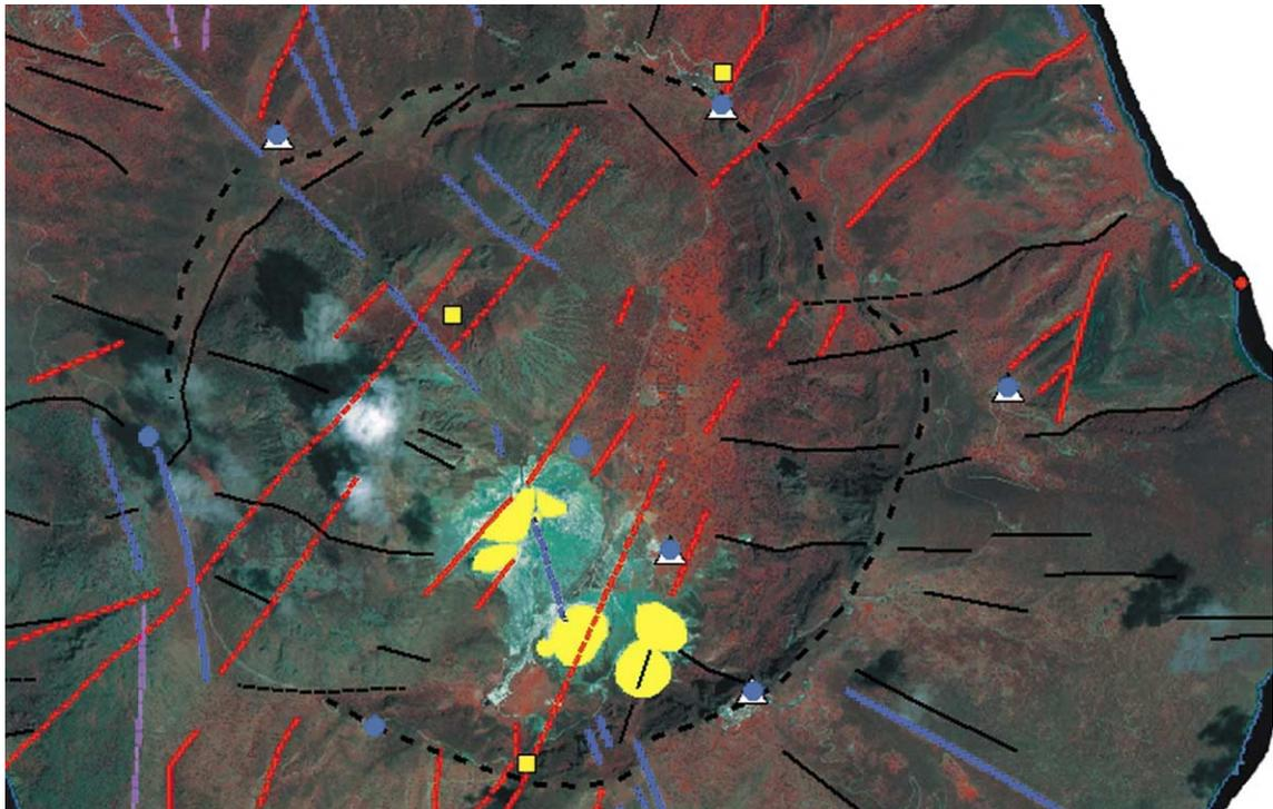
Fig. 9. The orthorectified IKONOS satellite image overlaid by the tectonic features (i.e. faults classified in categories, the position of GPS stations (blue circles), microgravimetric stations (triangles), fumaroles (squares)).
