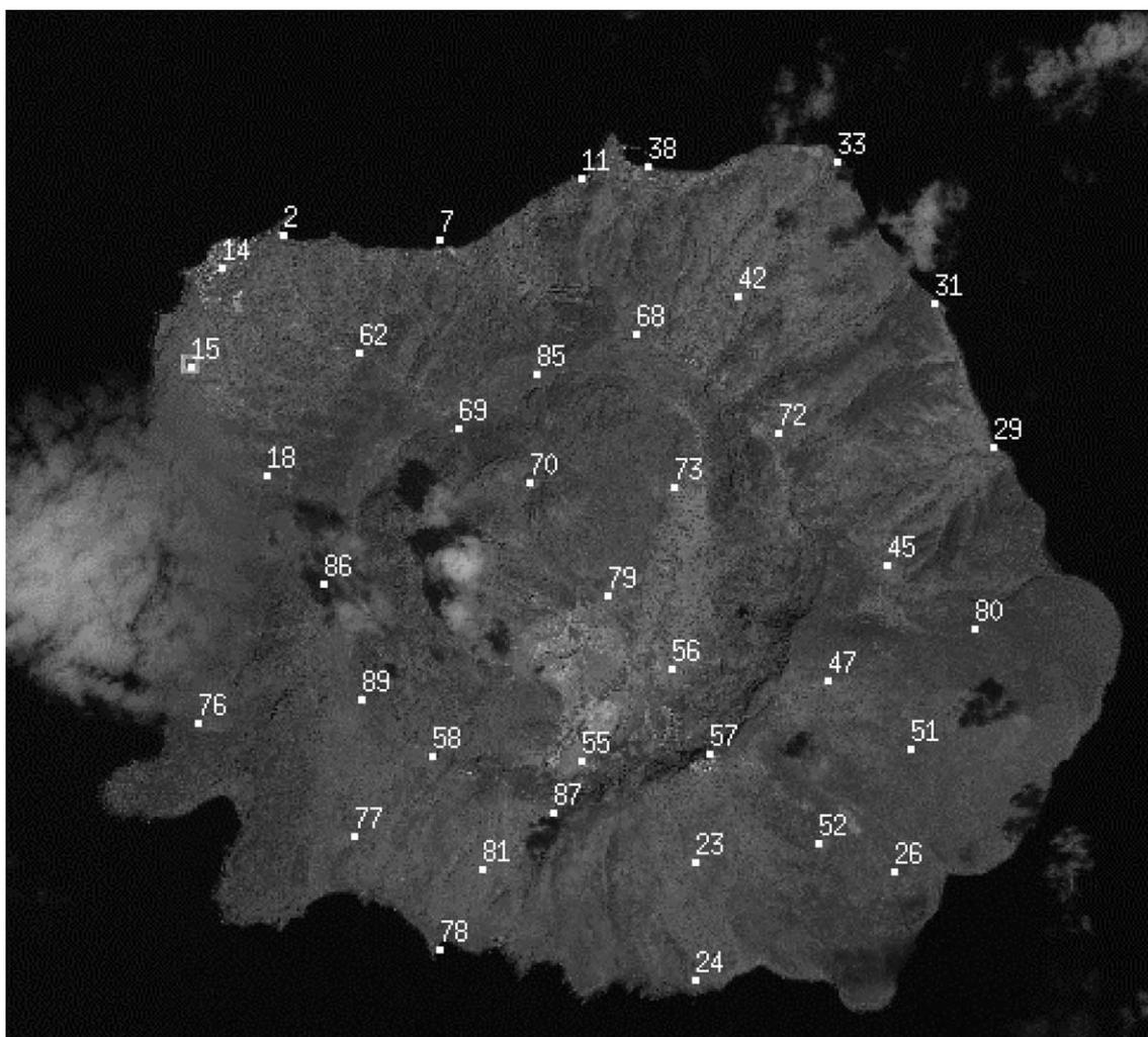
Fig. 2. IKONOS image of Nisyros Island with selected ground control points for orthorectification.
