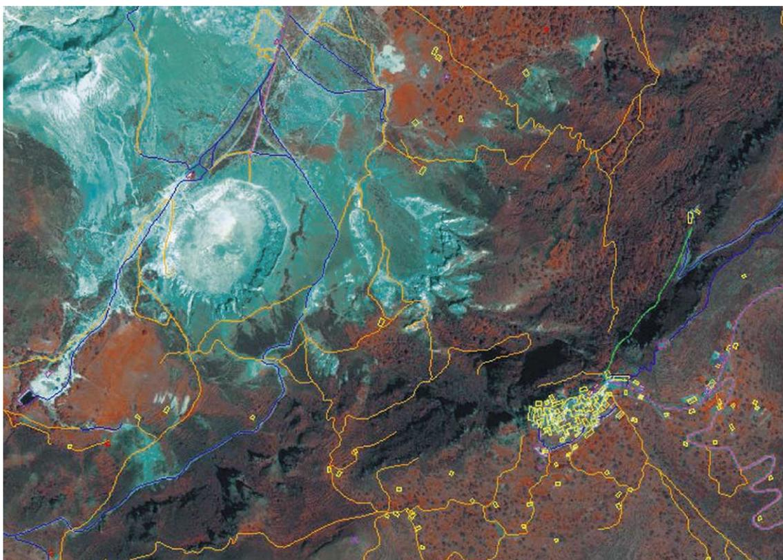
Fig. 8. The orthorectified IKONOS satellite image overlaid by the topographic information (roads, buildings, etc.) derived from field work and IKONOS. It represents a useful support for the topographic map update.
