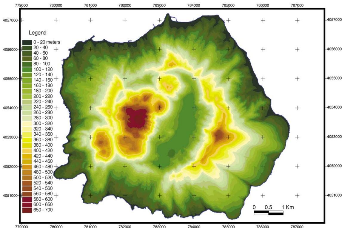
Fig. 4. The high-resolution DEM of Nisyros Island in grid format (cell size=2 m, Datum: Hellenic Geodetic Reference System 1987, Projection: TM).
