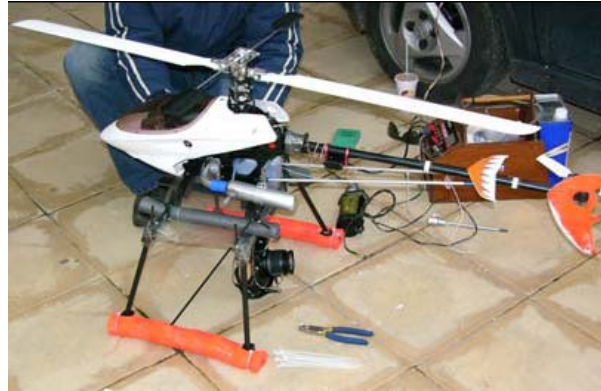
Figure 6: The camera mounting on the helicopter.
