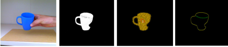
Fig. 1. Extracted image features. From left to right: the original image; the result of thresholding operations; pixel probabilities after labelling; resulting point features, where the contour is shown in yellow and the internal edge is depicted in green.
