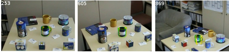
Fig. 5. Snapshot images with super imposed pose results from BoBoT’s ‘cup’ image sequence: MH3DOT tracker versus BLORT. The green line is the object pose from MH3DOT and the yellow line corresponds to BLORT.
