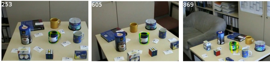
Fig. 5. Snapshot images with super imposed pose results from BoBoT’s ‘cup’ image sequence: MH3DOT tracker versus BLORT. The green line is the object pose from MH3DOT and the yellow line corresponds to BLORT.
