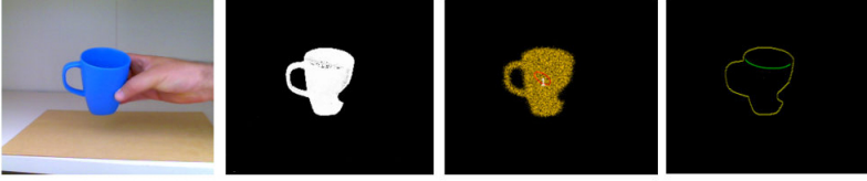
Fig. 1. Extracted image features. From left to right: the original image; the result of thresholding operations; pixel probabilities after labelling; resulting point features, where the contour is shown in yellow and the internal edge is depicted in green.
