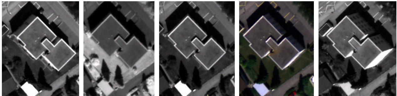
Figure 6. From left to right channel sequence: Backward, Near-infrared, Nadir, RGB, Forward. Geometric differences larger for backward and forward. Radiometric differences are large for near-infrared compared to other channels.
